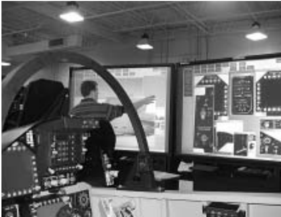
▲ F/A-18 Integrated Maintenance Training System built for the Canadian and Australian Forces, showing the replicated cockpit and two Interactive Panels.
