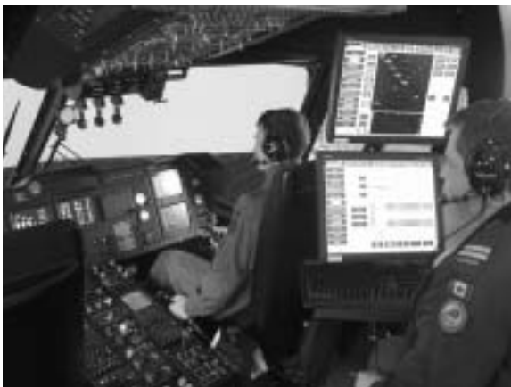
▲ Interior of the EH-101 helicopter Cockpit Procedures Trainer (CPT) developed for Westland Helicopters.
